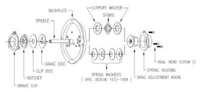
Drag Mechanism - Exploded View (Frame components removed for illustrative purposes )
